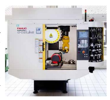
basic machine, a Robodrill  $\alpha$ -D21LiA5, which already has a very modest footprint. The three-axis standard Robodrill was upgraded by Häberle, using proven and standardised axes, to a five-axis machine. A side panel of the machine is removed, and a carousel especially developed and built by Häberle is mounted
